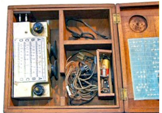
The receiver was carried in a wooden box with partitions for batteries and accessories.
