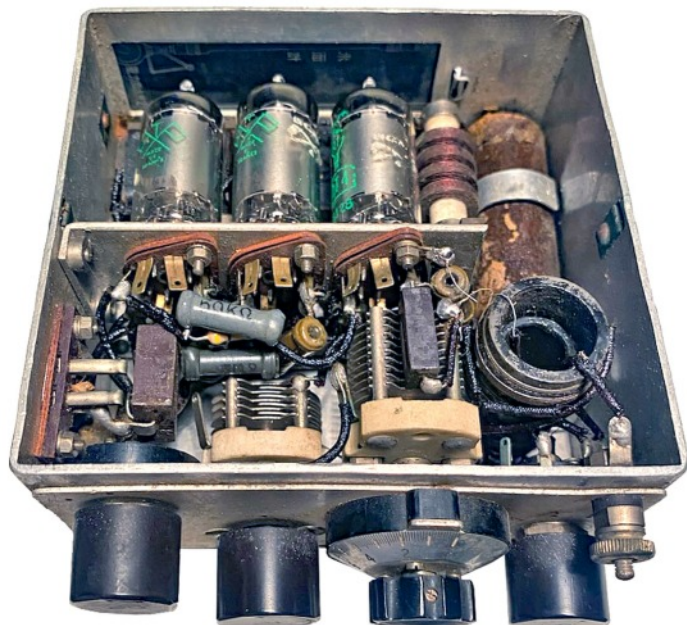
Components seen at the top side with cover detached. The valves shown here are modern 1T4 replacements to save the original WW2 originals during tests.
